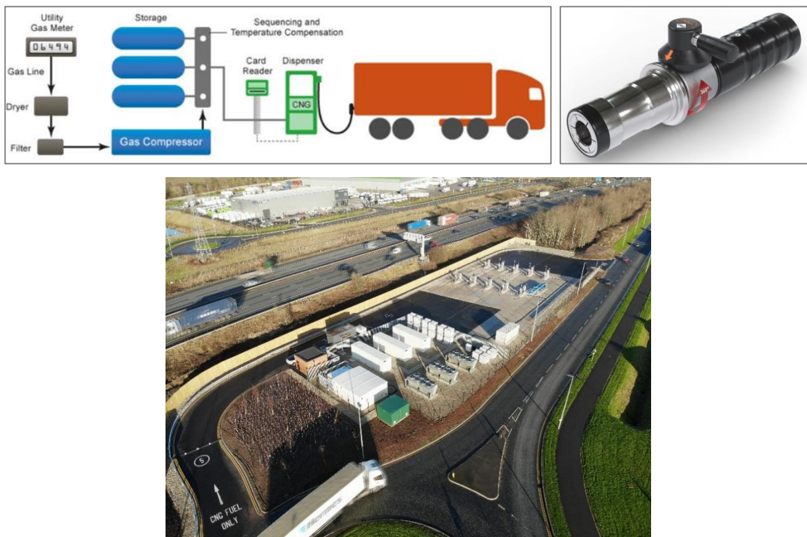
Figure 27 - Typical CNG Station Configuration (Source: US Environmental Protection Agency, Image: CNG Fuels Station, Warrington)
