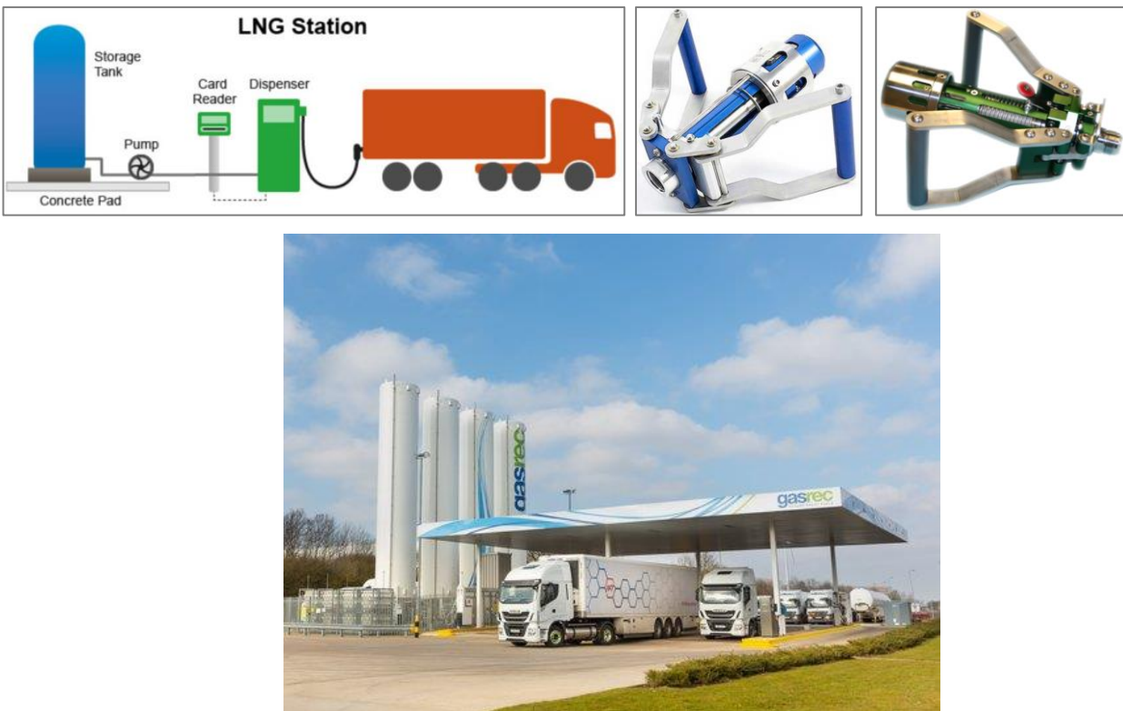
Figure 28 – Typical LNG Station Configuration (Source: US Environmental Protection Agency, Image: Gasrec Station, Daventry International Rail Freight Terminal)
